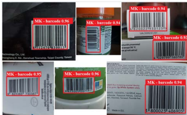
Fig. 1. Samples of successful barcode identification with YOLO-v5
